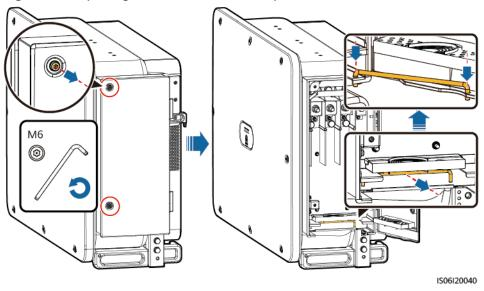
Figure 5-4 Opening the maintenance compartment door
