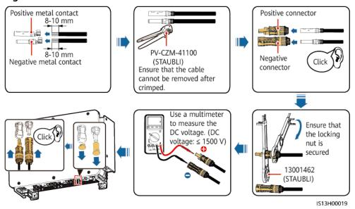
Figure 5-16 Connector connection
