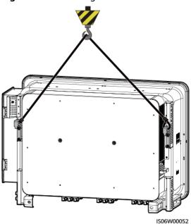
Figure 4-14 Hoisting the inverter
