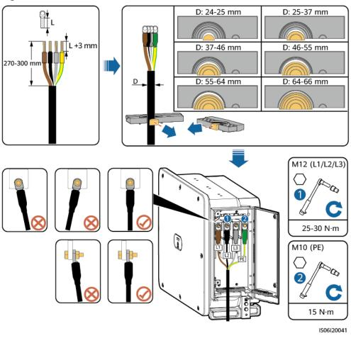
Figure 5-11 Cable connection
