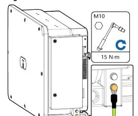
Figure 5-10 Cable connection
