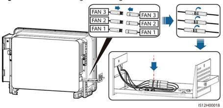
**Step 10** Push the fan tray into the slot and tighten the screw.
