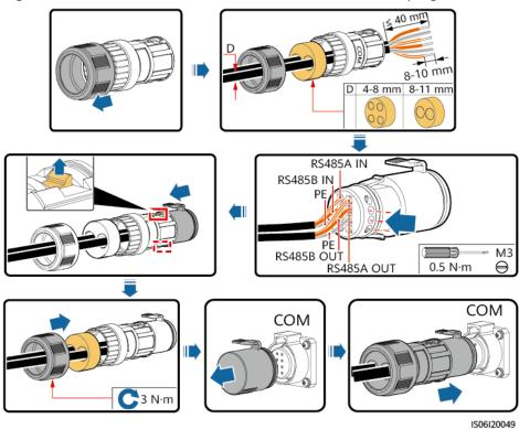
Figure 5-19 Cable connection (4-8 mm four-hole rubber plug)
