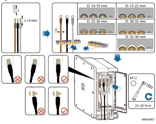
Figure 5-12 Cable connection
