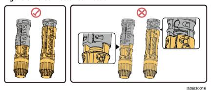
During DC input power cabling, leave at least 50 mm of slack. The axial tension on PV connectors must not exceed 80 N. Radial stress or torque must not be generated on PV connectors.
